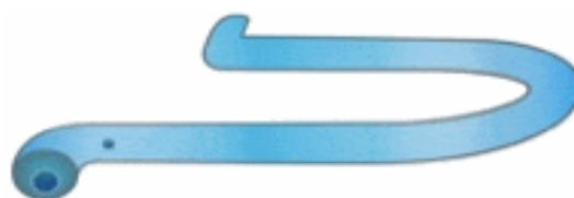
Fig.1. “Swinging” is generated by vibrating the tube(s) in which the fluid flows
